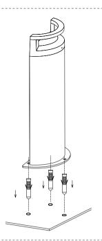
Drill holes according to base plate, insert plastic anchor into the holes.
