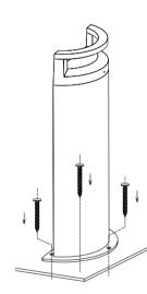
Lock the screw and fix the bollard.
